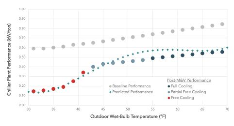
Our enhanced commissioning process delivered better than predicted performance in the  $45^{\circ}$  -  $55^{\circ}$  F wet bulb range.
