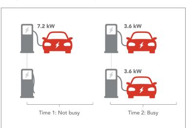
Figure 8. Illustration of atomated load management
